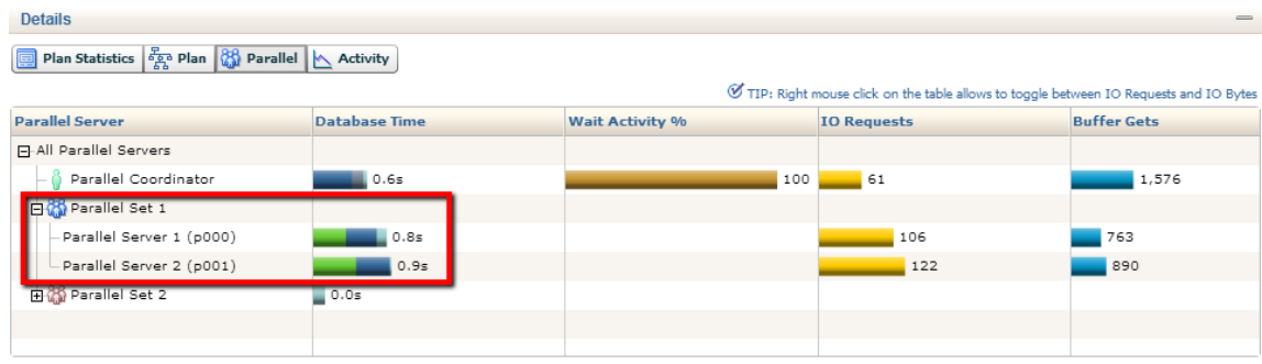
Figure 14-17. Showing the Parallel button page on the Details pane. Parallel Set 1 has been expanded
